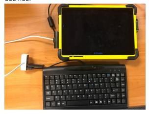
3. Power on the tablet. During power on, press keyboard "Esc" key several times to enter BIOS setup menu.
